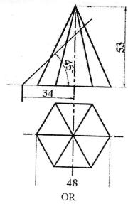
Draw the lines of intersection of the surfaces of geometrical solids shown in figure below. Also develop the lateral surface of the vertical solid.
